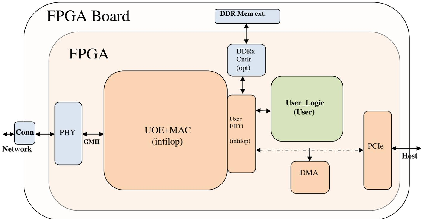
**FPGA Development System with fully integrated and tested;
