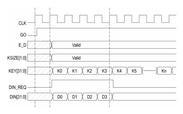
The KSIZE parameter is passed to the core when GO signal is raised.
