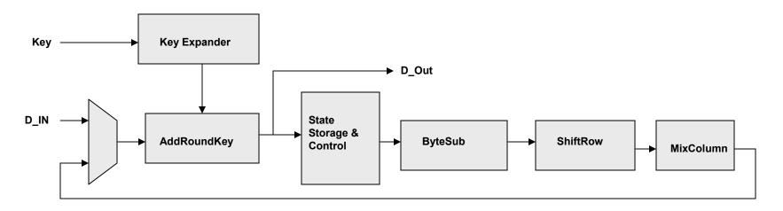
•Data\_In and the key are added together in the AddRoundKey module
