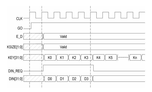
The KSIZE parameter is passed to the core when GO signal is raised. Input of the KEY data continues for the duration of the cryptographic operation. Both the data and the key are input serially, 32 bits at a time. Diagram above shows the case where the input data is 128 bits.
