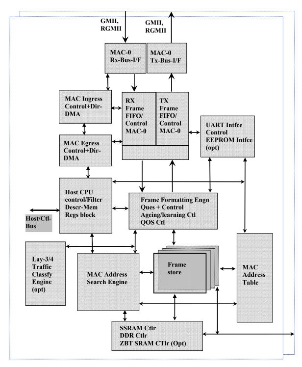
Giga-bit Multi-port Switch Architecture
